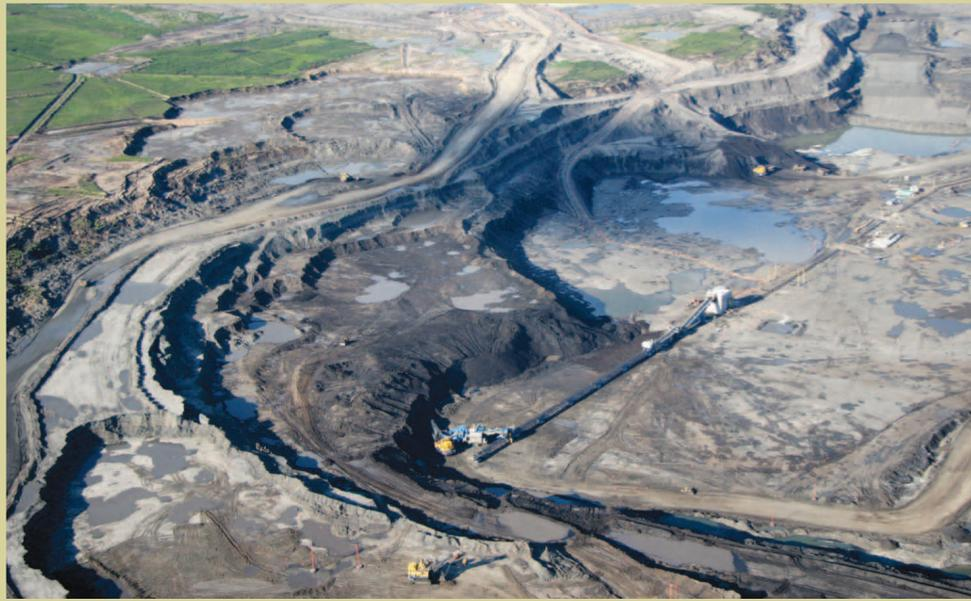
2008, Alberta, Canada. Aerial photo of massive open pit mines to get to oil sands and the production of a tar-like form of petroleum. The petroleum requires either strip mining or using large amounts of steam and solvents to force it to flow to wells. Tar-sands oil extraction produces three times more greenhouse gas than conventional oil production, causing vast destruction of forests and spoiling ecosystems.
